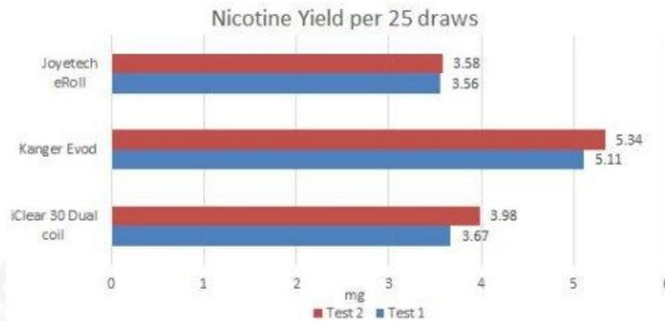
Vapour was collected from the three devices using a protocol that approximated the inhalation volume of experienced e-cigarette users. Samples were collected using an analytical smoking machine set to deliver a 55 ml 4 second puff every 30 seconds. 200 puffs were collected per device in blocks of 25 puffs. From this data, it is possible to determine the amount of nicotine delivered on a per puff basis.
