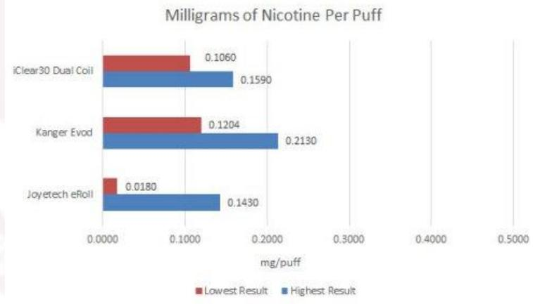
The above graph shows the total amount of nicotine produced during a 55ml 4 second draw. The highest and lowest results were taken from both test runs to show the variation in nicotine delivery. The Joyetech eRoll has a higher variation due to voltage drop on its small 90mah battery.
